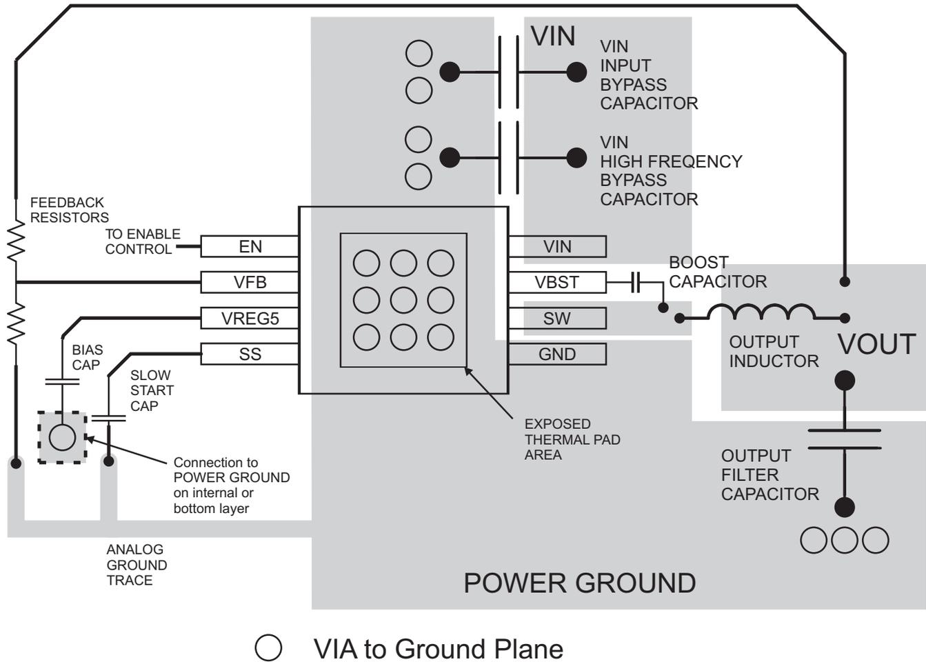
Figure 16. PCB Layout
