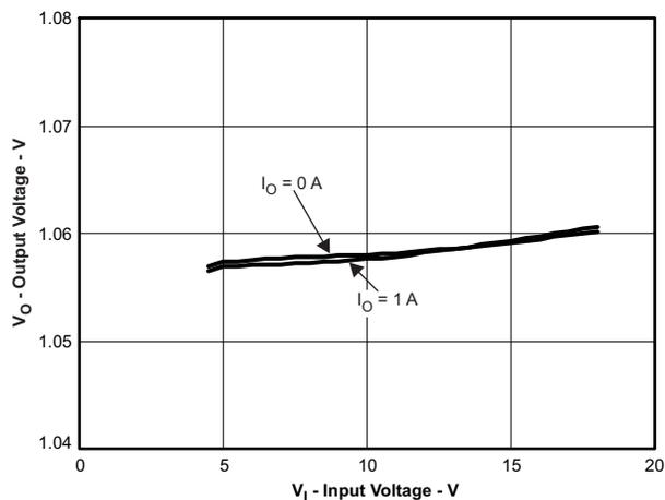
Figure 5. 1.05-V OUTPUT VOLTAGE vs INPUT VOLTAGE
