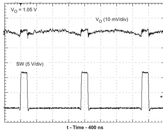
**Figure 12. VOLTAGE RIPPLE AT OUTPUT (IO = 2 A)**
