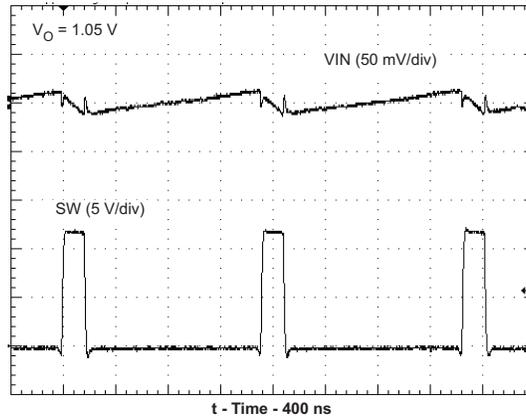
**Figure 13. VOLTAGE RIPPLE AT INPUT ( $I_O = 2\text{ A}$ )**
