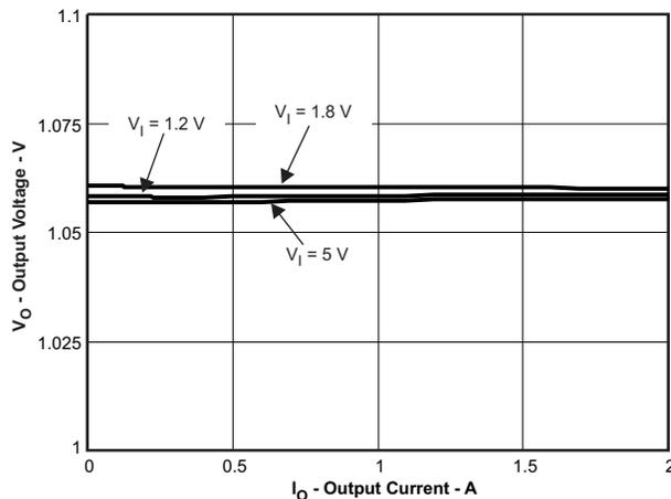
Figure 4. 1.05-V OUTPUT VOLTAGE vs OUTPUT CURRENT
