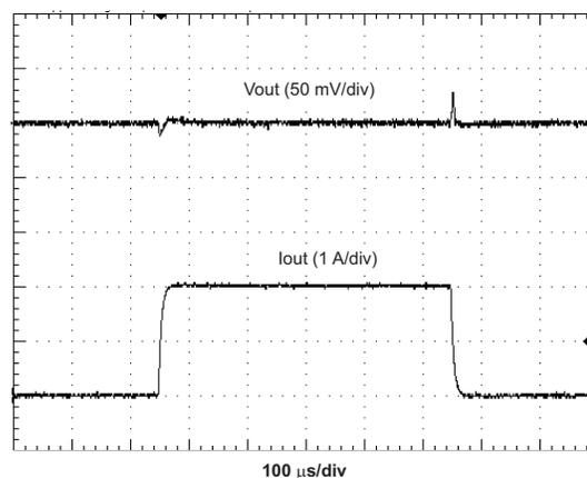
Figure 6. 1.05-V, 0-A to 2-A LOAD TRANSIENT RESPONSE
