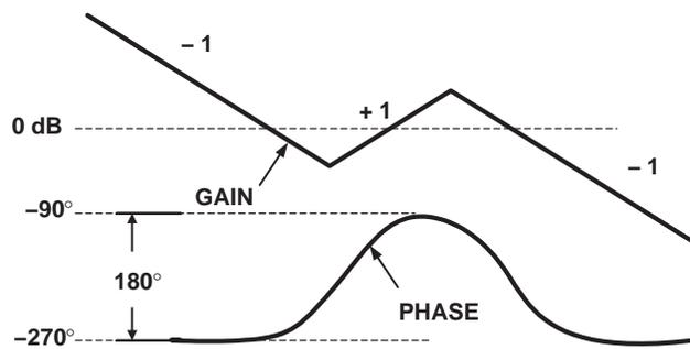
Figure 8. Type III Compensation Gain and Phase
