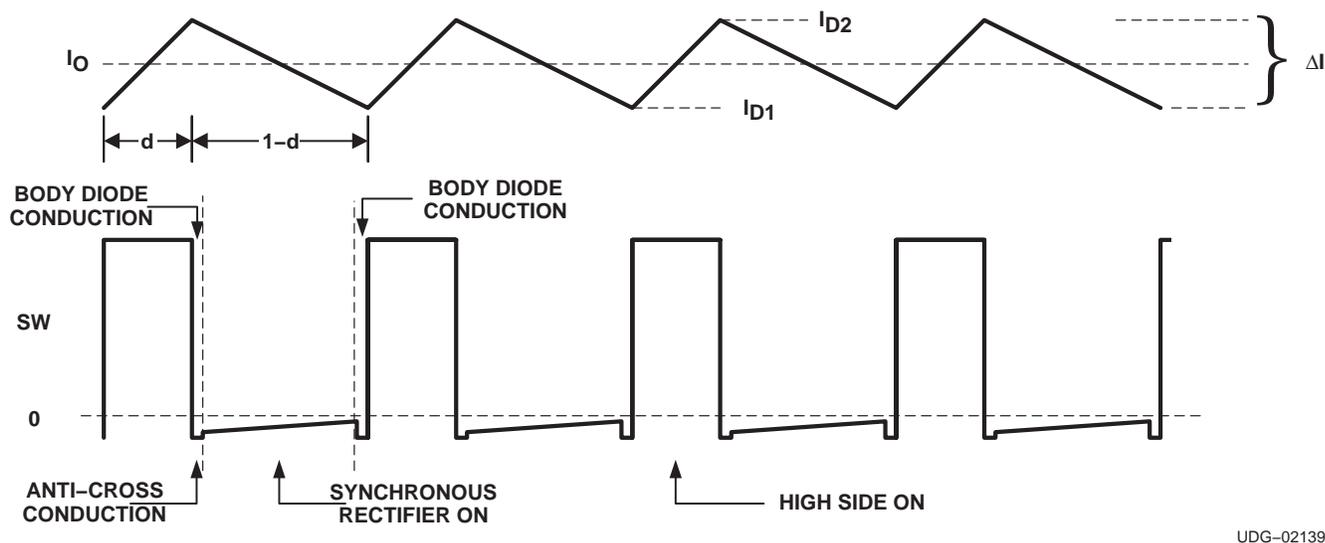
Figure 9. Inductor Current and SW Node Waveforms
