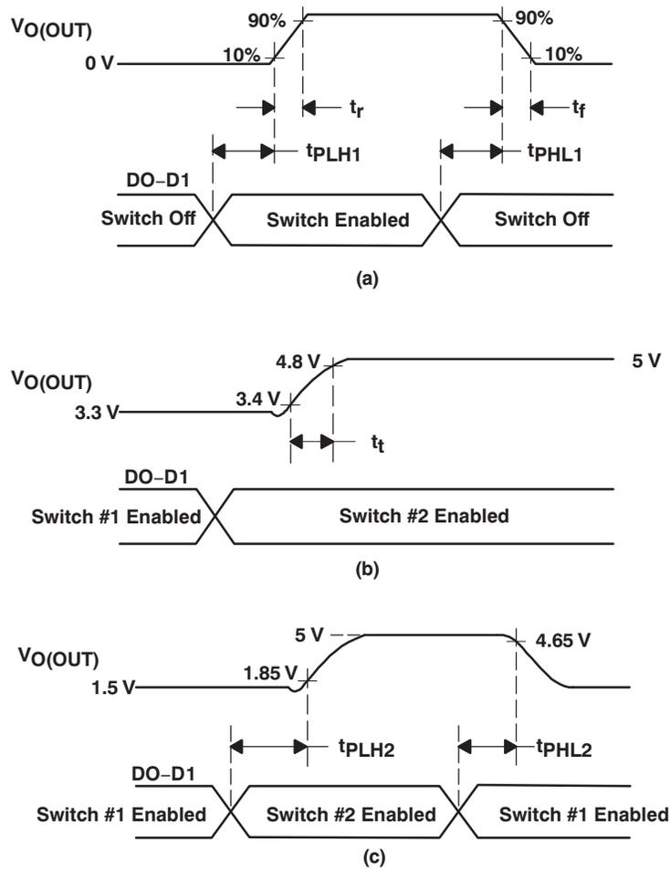
**Figure 1. Propagation Delays and Transition Timing Waveforms**
