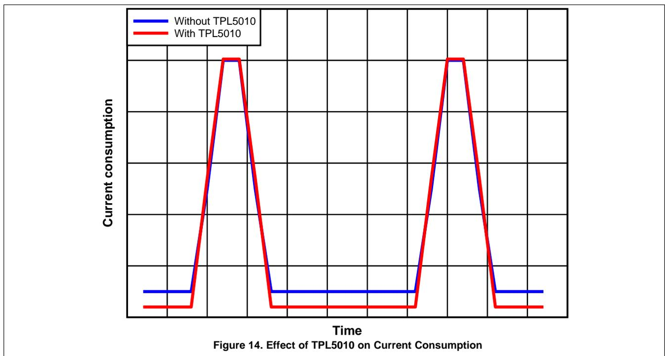
Figure 14. Effect of TPL5010 on Current Consumption
