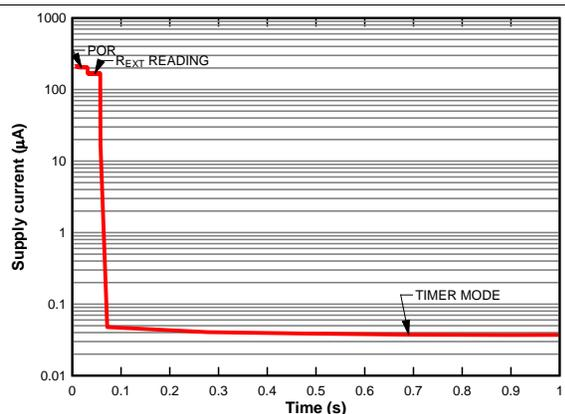
Figure 6.  $I_{DD}$  vs. Time
