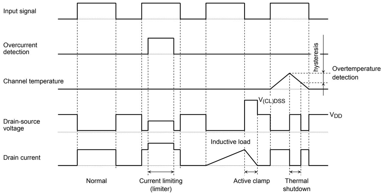
Note 2: The overtemperature detector circuits feature hysteresis. After overtemperature is detected, normal operation is restored only when the channel temperature falls by the hysteresis amount (5°C typ.) in relation to the overtemperature detection temperature.
