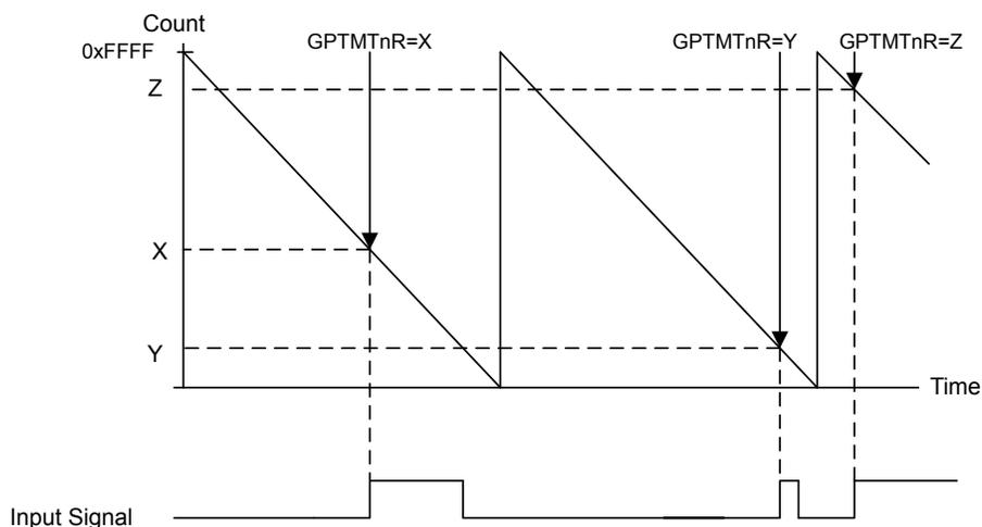
**Note:** When operating in Edge-time mode, the counter uses a modulo  $2^{24}$  count if prescaler is enabled or  $2^{16}$ , if not. If there is a possibility the edge could take longer than the count, then another timer configured in periodic-timer mode can be implemented to ensure detection of the missed edge. The periodic timer should be configured in such a way that:
