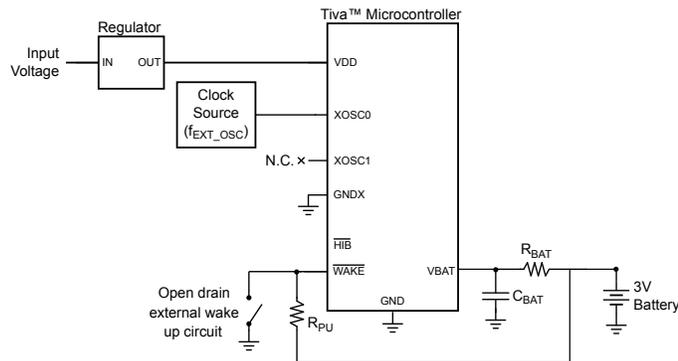
**Note:** Some devices may not supply the GNDX,  $\overline{\text{WAKE}}$  or  $\overline{\text{HIB}}$  signals. See “Signal Tables” on page 1224 for pins specific to your device.
