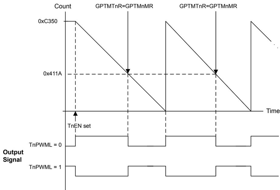
When synchronizing the timers using the **GPTMSYNC** register, the timer must be properly configured to avoid glitches on the CCP outputs. Both the  $TnPLO$  and the  $TnMRSU$  bits must be set in the **GPTMTnMR** register. Figure 11-6 on page 717 shows how the CCP output operates when the  $TnPLO$  and  $TnMRSU$  bits are set and the **GPTMTnMATCHR** value is greater than the **GPTMTnILR** value.
