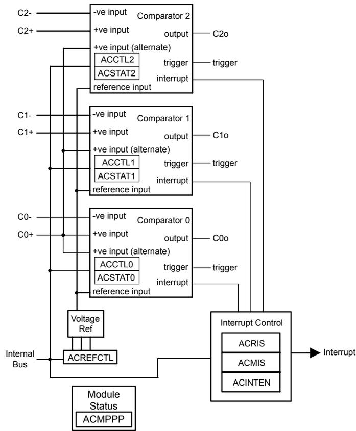
**Note:** This block diagram depicts the maximum number of analog comparators and comparator outputs for the family of microcontrollers; the number for this specific device may vary. See page 1120 for what is included on this device.
