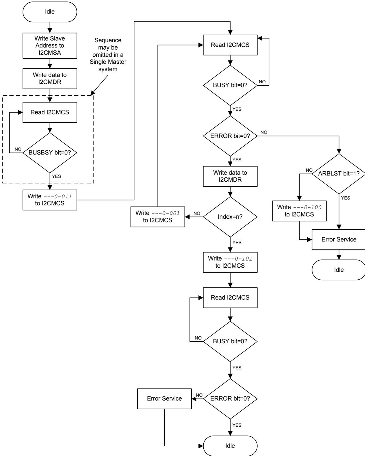
Figure 16-11. Master RECEIVE of Multiple Data Bytes
