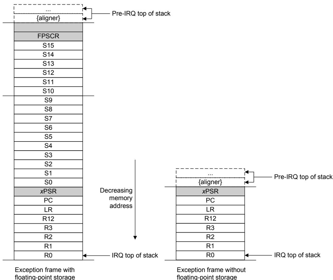
Immediately after stacking, the stack pointer indicates the lowest address in the stack frame.
