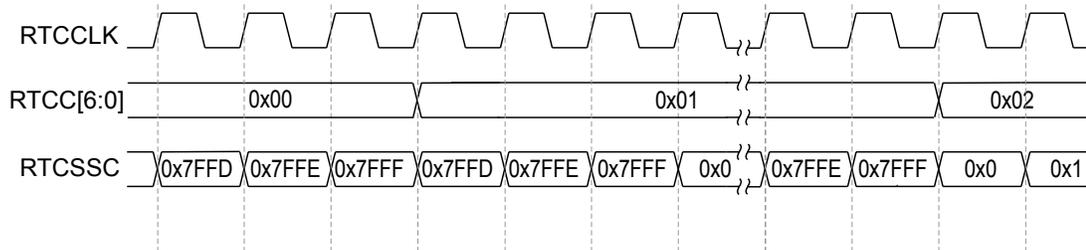
In the case of a trim value below `0x7FFF`, the `RTCSSC` value is advanced from `0x7FFF` to the trim value while the `RTCC` value is incremented from `0x0` to `0x1`. If the match value is within that range, the match interrupt is not triggered. For example, as shown in Figure 7-6 on page 496, if the match interrupt was configured with `RTCM0=0x1` and `RTCSSM=0x2`, an interrupt would never be triggered.
