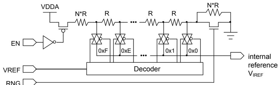
**Note:** In the figure above,  $N \cdot R$  represents a multiple of the  $R$  value that produces the results specified in Table 18-2 on page 1109.
