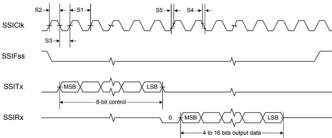
Figure 23-22. Master Mode SSI Timing for SPI Frame Format (FRF=00), with SPH=1
