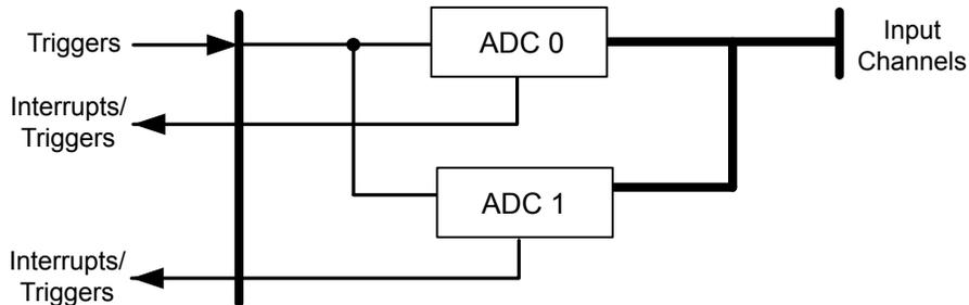
Figure 13-2 on page 801 provides details on the internal configuration of the ADC controls and data registers.
