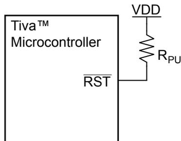
$R_{\text{PU}} = 0$  to 100 k $\Omega$
