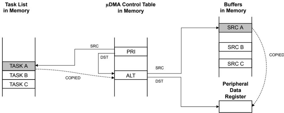
Using the channel's primary control structure, the  $\mu$ DMA controller copies task A configuration to the channel's alternate control structure.
