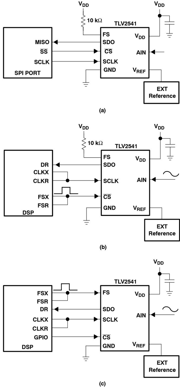
**Figure 29. Typical TLV2541 Interface to a TMS320 DSP**
