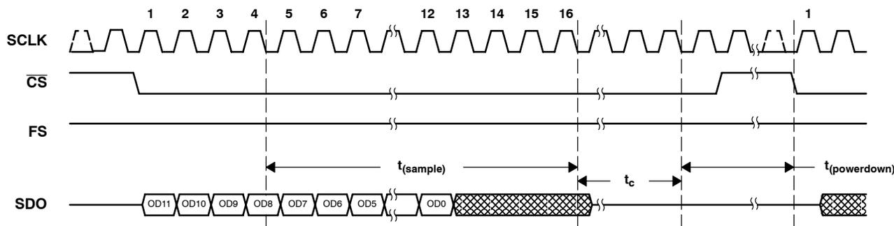
**Figure 2. TLV2541 Timing: Control via  $\overline{CS}$  (FS = 1)**
