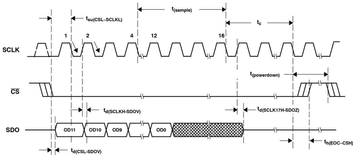
**Figure 7. TLV2541 Critical Timing (Control via  $\overline{CS}$  only, FS = 1)**
