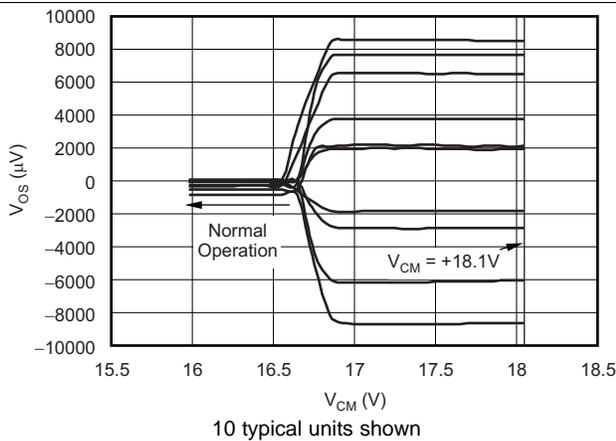
Figure 3. Offset Voltage vs Common-Mode Voltage (Upper Stage)
