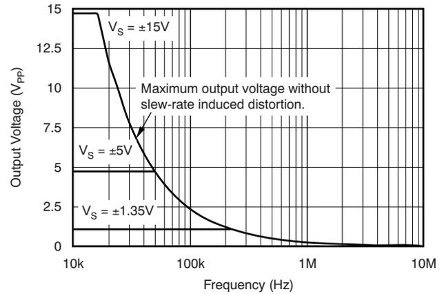
Figure 24. Maximum Output Voltage vs Frequency
