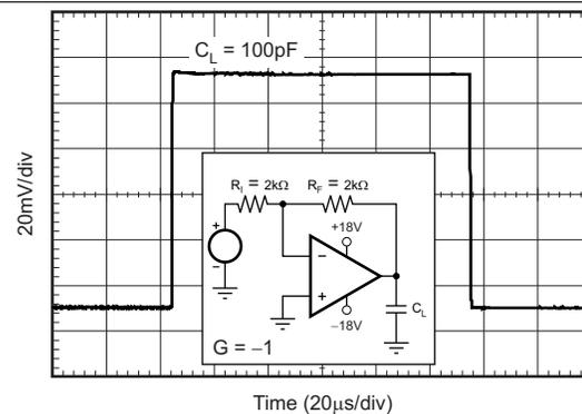
Figure 18. Small-Signal Step Response (100 mV)
