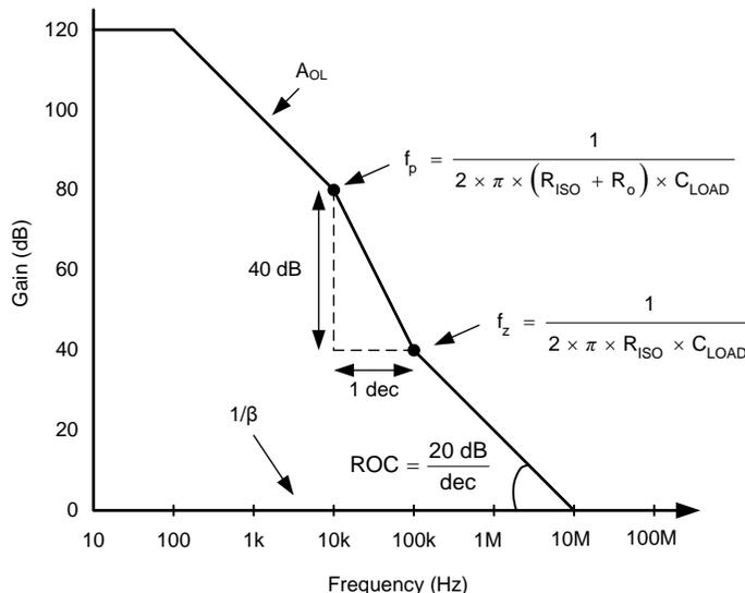
Figure 31. Unity-Gain Amplifier With R<sub>ISO</sub> Compensation
