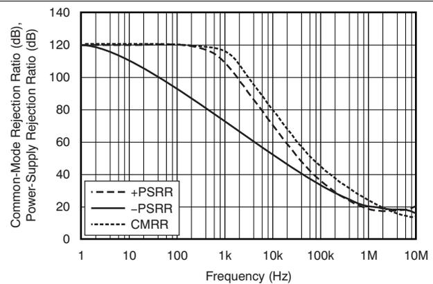
Figure 6. CMRR and PSRR vs Frequency (Referred-to Input)
