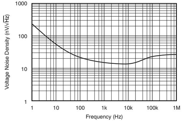
Figure 8. Input Voltage Noise Spectral Density vs Frequency
