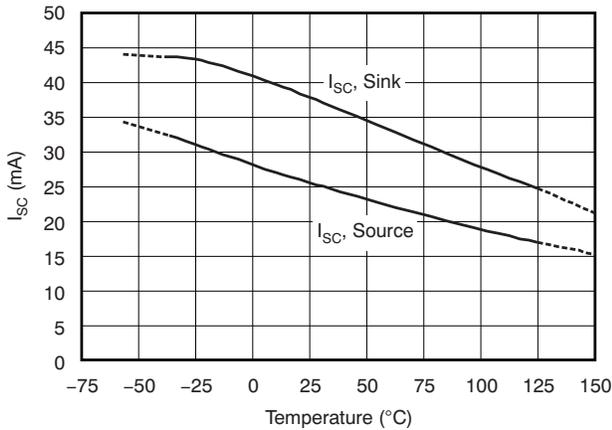
Figure 23. Short-Circuit Current vs Temperature
