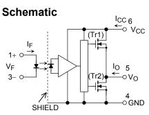
A 0.1- $\mu$ F bypass capacitor must be connected between pins 6 and 4. (See Note 6.)
