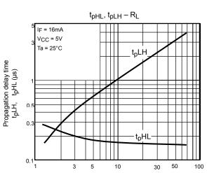
Load resistance  $R_L$   $(k\Omega)$
