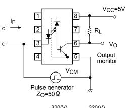
$$\text{CM}_{H} = \frac{320(\text{V})}{t_{\text{\Gamma}}(\mu s)}, \text{CM}_{L} = \frac{320(\text{V})}{t_{\text{f}}(\mu s)}$$
