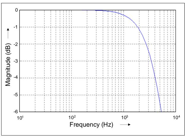
Figure 7 DAC Input Filter (Magnitude Plot)
