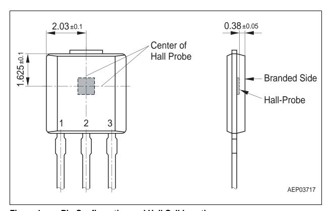
Figure 1 Pin Configuration and Hall Cell Location
