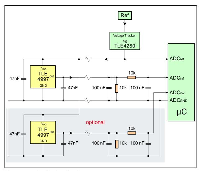
Figure 10 Application Circuit
