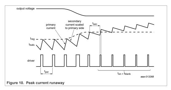
The output voltage can drop, for instance, because a load is too high or a short-circuit event occurs. If the output voltage drops, the decrease of the transformer current during the secondary stroke time ( $t_{sec}$ ) becomes less. As a result, the next cycle starts at a higher peak current.
