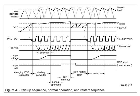
When the voltage on pin VCC drops to below the  $V_{th(UVLO)}$  level during normal operation, the controller stops switching. The TEA1833TS waits for the rectified mains to charge the VCC pin to  $V_{startup}$  using resistor R1.
