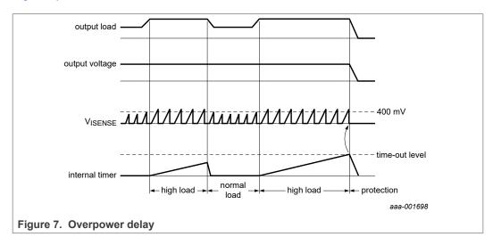
When the overload timeout is reached, the TEA1833TS enters the overpower restart mode. In overpower restart mode, the VCC capacitor is discharged to UVLO level and then charged to the start-up level three times before the converter switches again.
