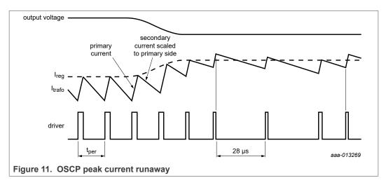
If the system detects that the peak current already exceeds the targeted level after 1  $\mu$ s, the next switching period time is extended from 7.7  $\mu$ s (f<sub>sw</sub> = 130 kHz) to 28  $\mu$ s (f<sub>sw</sub> = 36 kHz). The time of the secondary stroke is then sufficient to decrease the transformer current to below the targeted peak current again.
