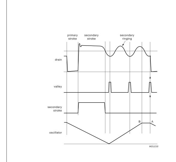
A: Start of new cycle at lowest drain voltage.
