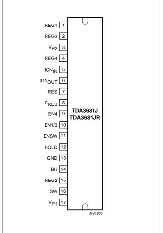
Fig.3 Pin configuration for TDA3681J and TDA3681JR.
