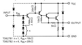
Note: The input and output parasitic diodes cannot be used as clamp diodes.
