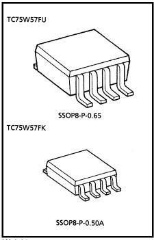
Weight SSOP8-P-0.65: 0.021g (typ.) SSOP8-P-0.50A: 0.01g (typ.)
