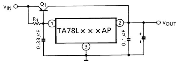
Use a required radiation plate for Q<sub>1</sub>.
