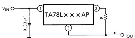
$$I_{OUT} = \frac{V_{OUT}}{R} + I_B$$
