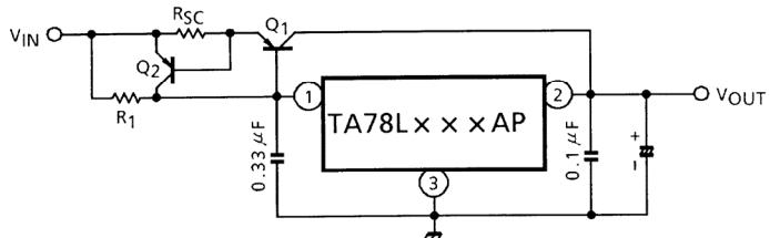
$$R_{SC} = \frac{V_{BE2}}{I_{SC}}$$
