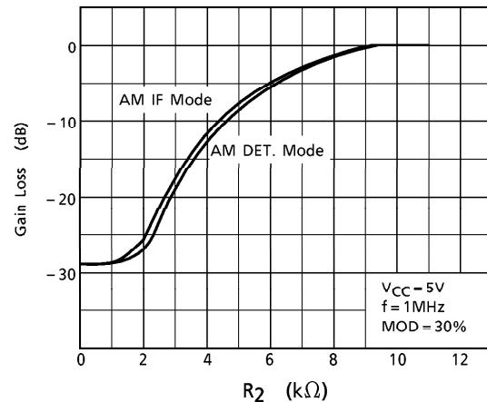
(Note) It is necessary to set up the value of R<sub>2</sub> under 20kΩ.
