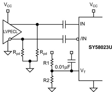
For V<sub>CC</sub> = 2.5V, R<sub>pd</sub> = 50Ω, R1 = 1k, R2 = 1.1k Ω.
