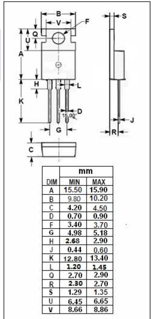
**High Voltage Power Schottky Rectifier****STPS20H100CT****THERMAL CHARACTERISTICS**
