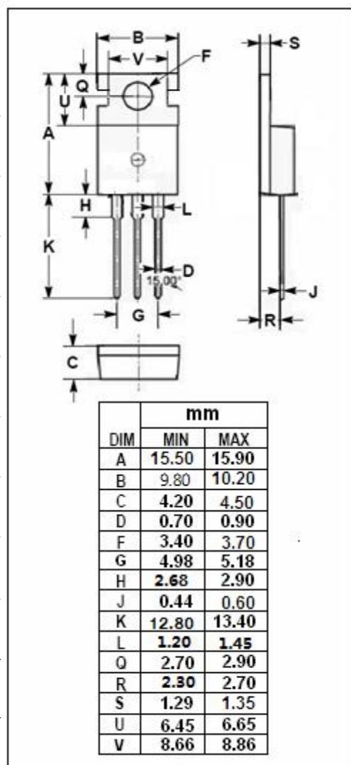
**Isc N-Channel MOSFET Transistor****STP57N65M5****ELECTRICAL CHARACTERISTICS**T<sub>c</sub>=25°C unless otherwise specified
