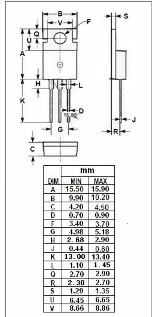
**Isc N-Channel MOSFET Transistor**
