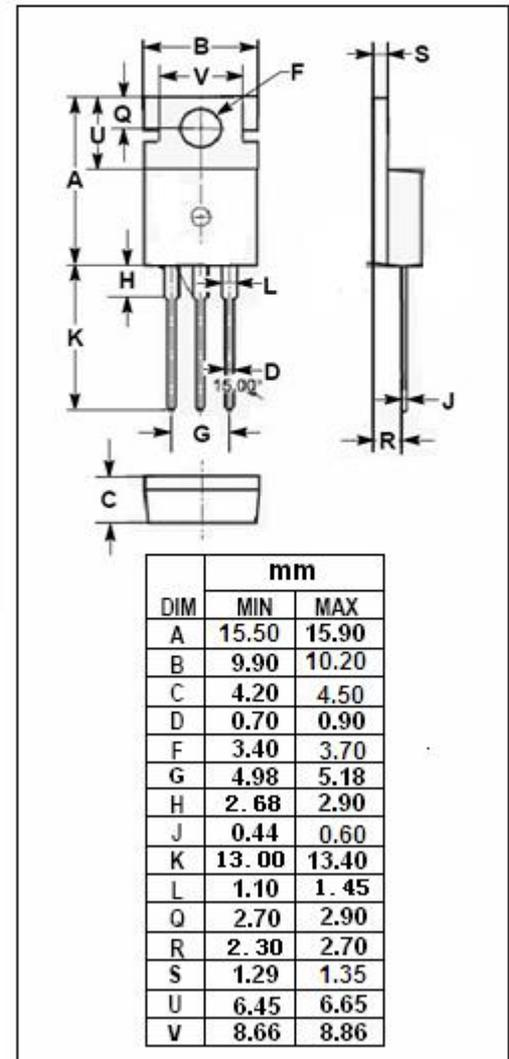
**Isc N-Channel MOSFET Transistor**
