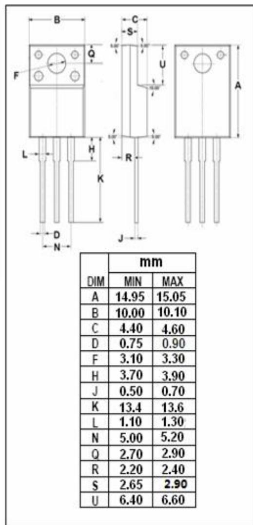
**Isc N-Channel MOSFET Transistor****STP10NK60ZFP****ELECTRICAL CHARACTERISTICS** $T_c=25^\circ\text{C}$  unless otherwise specified
