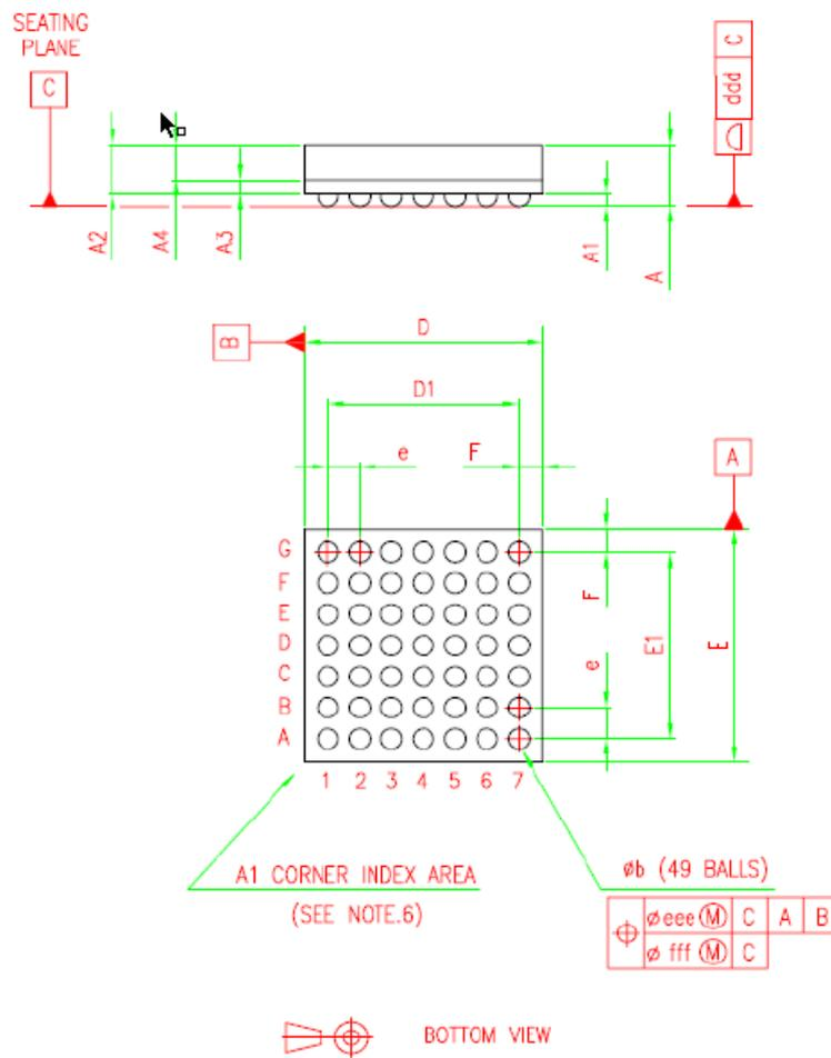
**Note:** The terminal A1 corner must be identified on the top surface by using a corner chamfer, ink or metallized marking, or other feature of package body or integral heatslug. A distinguishing feature is allowed on the bottom surface of the package to identify the terminal A1 corner. Exact shape of each corner is optional.
