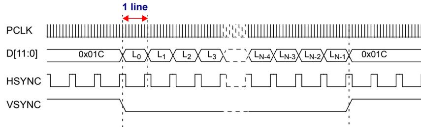
Figure 5. 12-bit parallel data interface signals - line level
