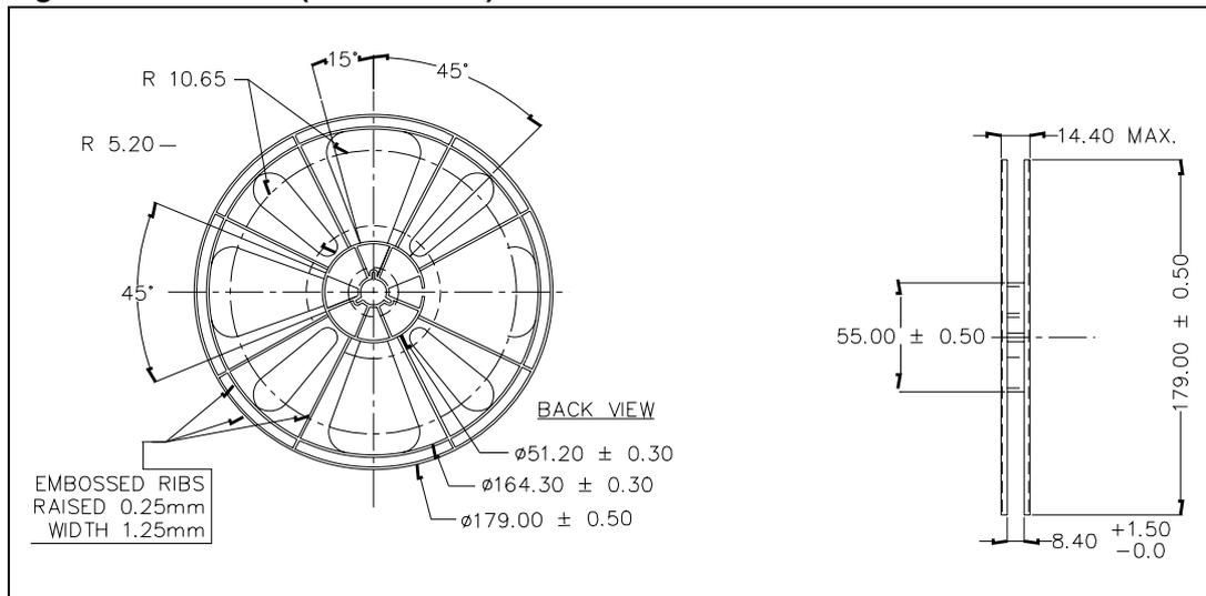
Figure 16. QFN10L (1.8 x 1.4 mm) reel information - front side
