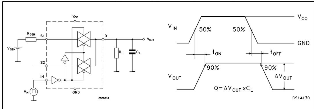
**Figure 11. Turn on, turn off delay time**
