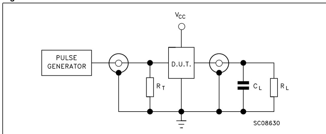
1.  $C_L = 5/35\ \text{pF}$  or equivalent (includes jig and probe capacitance)
