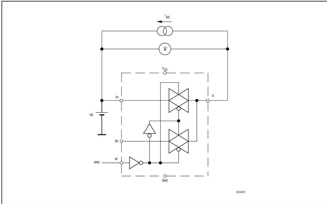
Figure 4. OFF leakage
