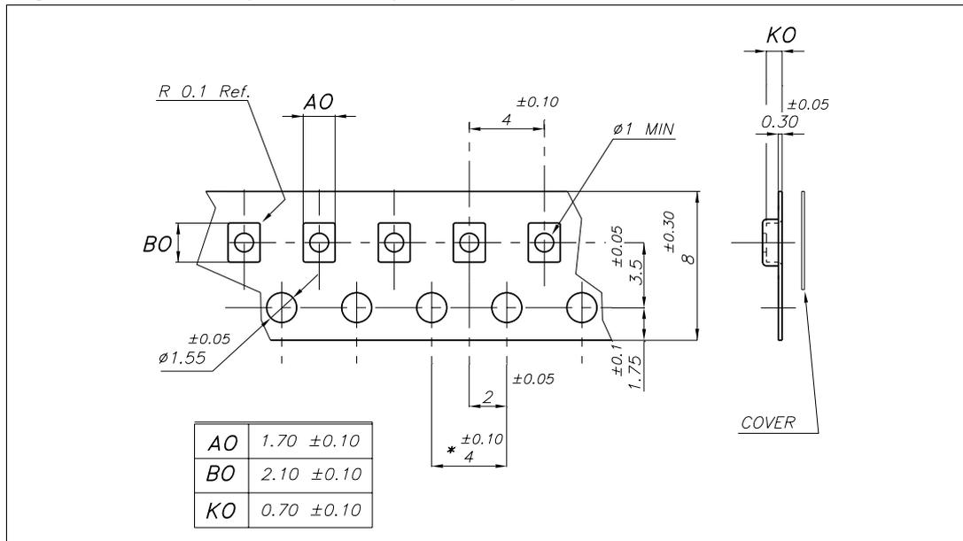
Figure 15. QFN10L (1.8 x 1.4 mm) reel information - back view
