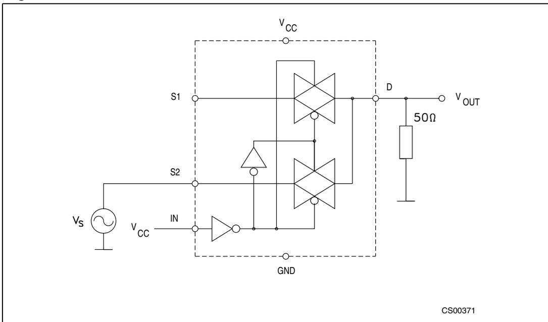
Figure 7. Channel-to-channel crosstalk
