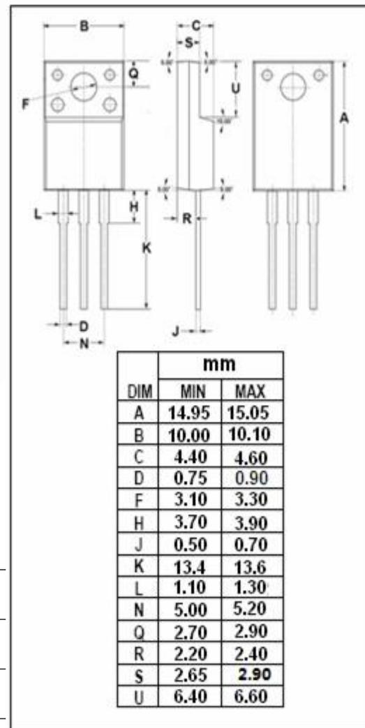
**Isc N-Channel MOSFET Transistor****STF23NM50N****ELECTRICAL CHARACTERISTICS**T<sub>C</sub>=25°C unless otherwise specified
