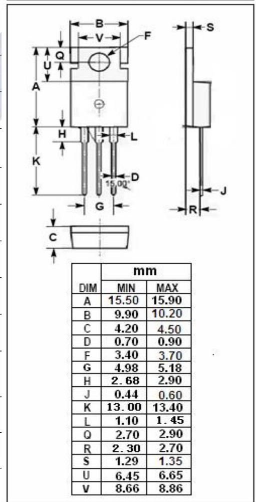
**isc P-Channel MOSFET Transistor**
