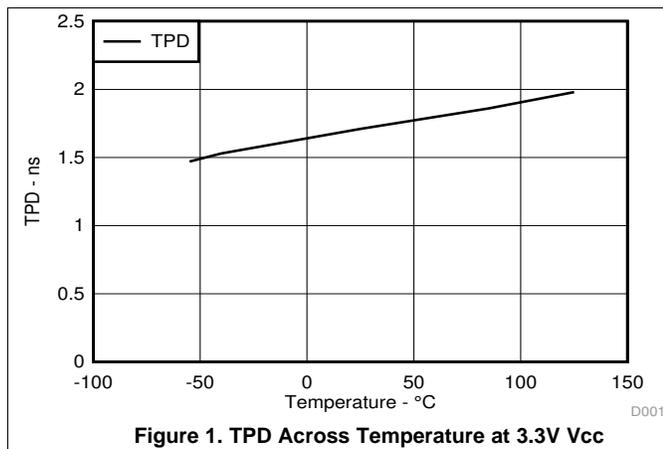
Figure 1. TPD Across Temperature at 3.3V Vcc
