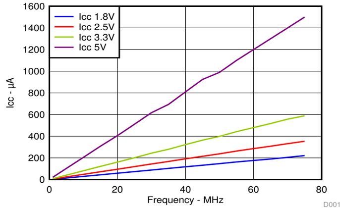
Figure 6. I<sub>CC</sub> vs Frequency
