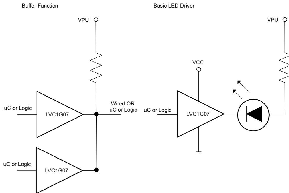
**Figure 5. Typical Application-SN74LVC1G07-Q1**
