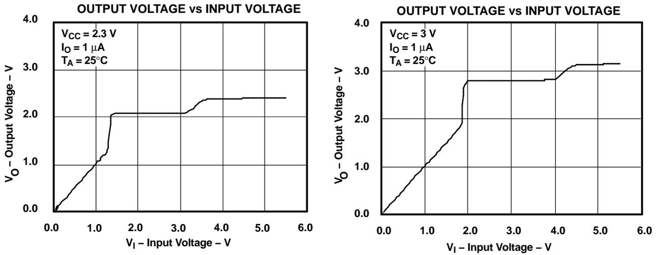
Figure 3. Data Output Voltage vs Data Input Voltage
