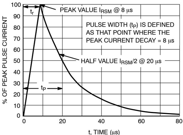
**Figure 3. 8 x 20 μs Pulse Waveform**
