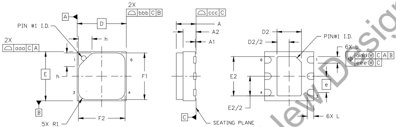
Figure 8. 3x3 6-pin DFN with Protective Cover
