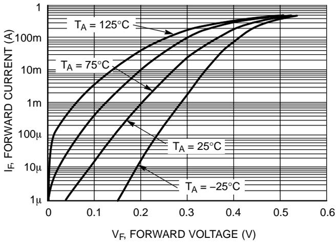
**Figure 1. Forward Characteristics**
