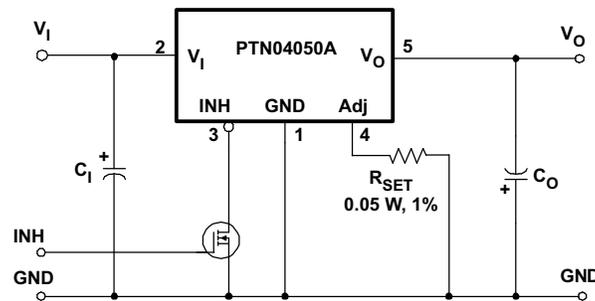
Figure 17. Inhibit Circuit
