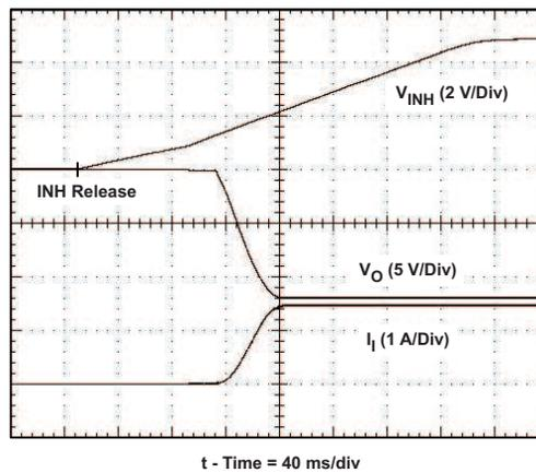
Figure 18. Inhibit Waveform
