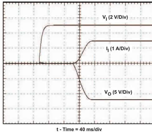
Figure 16. Power-Up Waveforms
