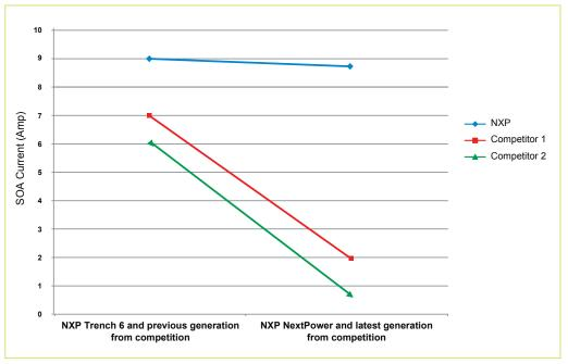
Condition: SOA Drain current (Amp) @  $V_{ds}$ =10 V, 10 ms pulse for a 5 m $\Omega$  (@ 10 V) in Power SO8
