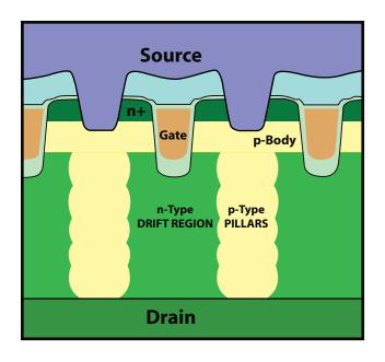
NextPower technology uses p-Type pillars to improve the breakdown voltage in the OFF state, and a heavily doped n-Type drift region to achieve exceptionally low ON resistance.
