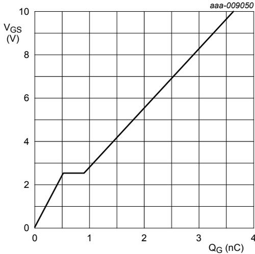
$I_D = 3.2 \text{ A}; V_{DS} = 15 \text{ V}; T_{amb} = 25 \text{ }^\circ\text{C}$
