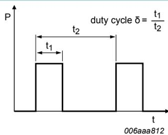
Fig. 18. Duty cycle definition
