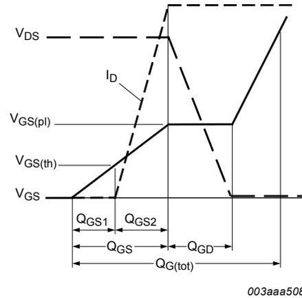
Fig. 16. MOSFET transistor: Gate charge waveform definitions
