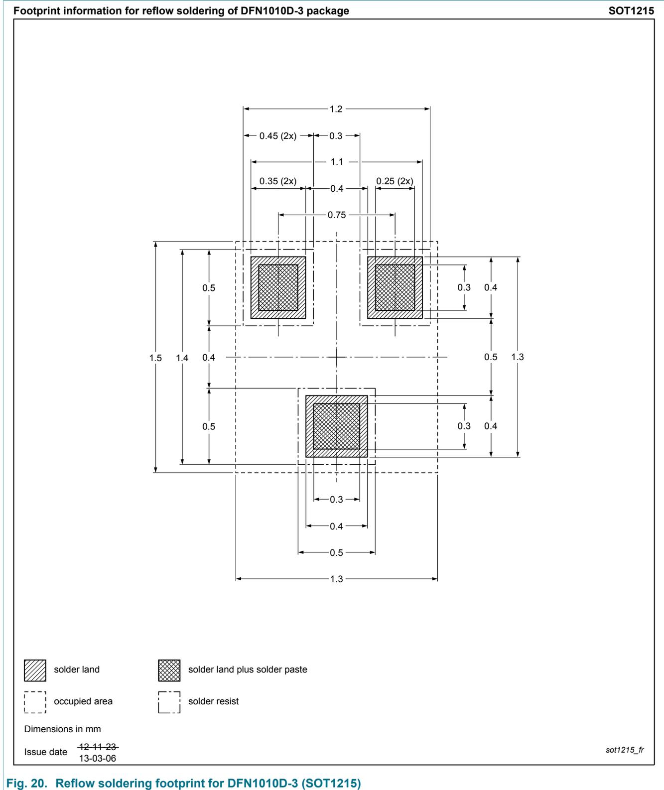
Fig. 20. Reflow soldering footprint for DFN1010D-3 (SOT1215)
