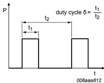
Fig. 18. Duty cycle definition
