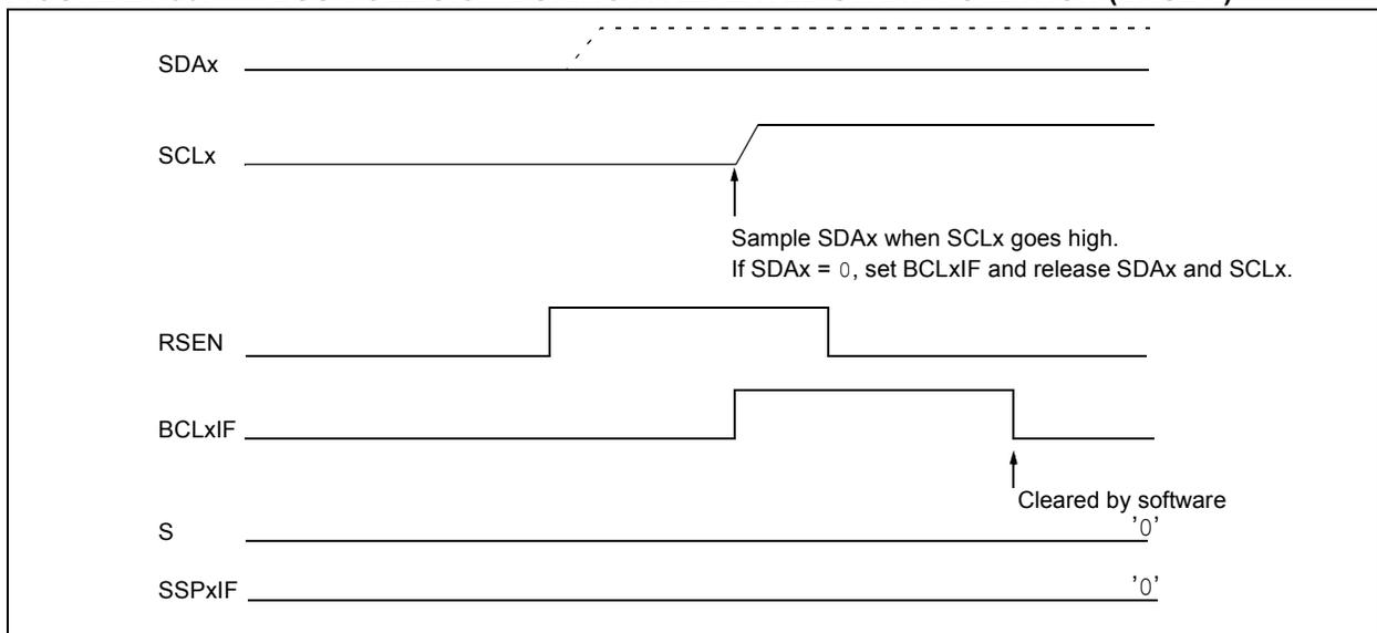
**FIGURE 24-37: BUS COLLISION DURING REPEATED START CONDITION (CASE 2)**
