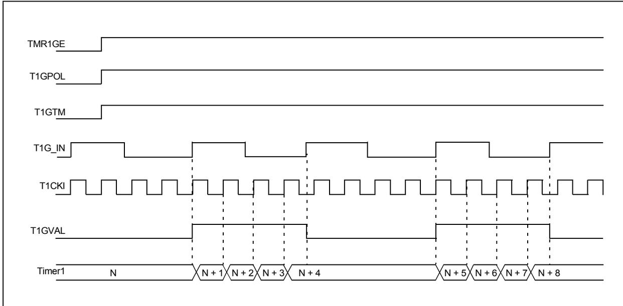
**FIGURE 20-5: TIMER1 GATE SINGLE-PULSE MODE**
