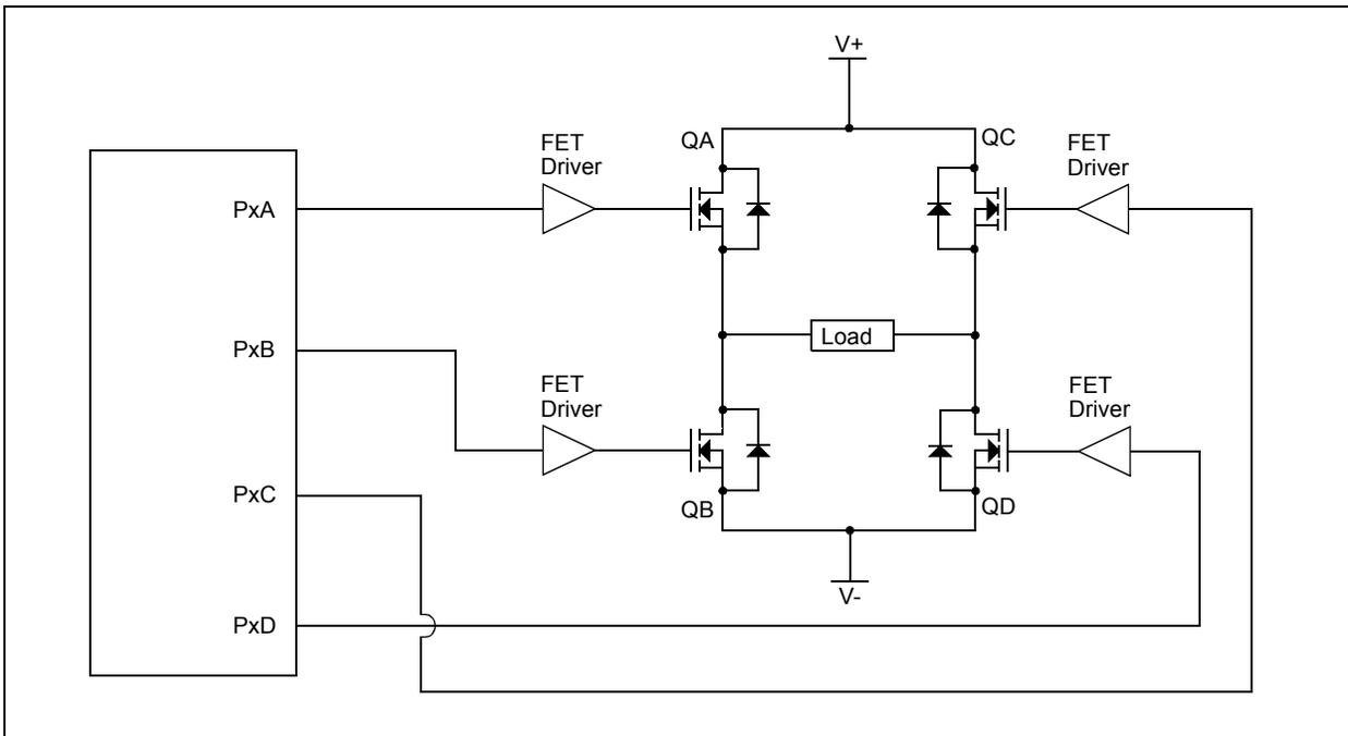
**FIGURE 23-11: EXAMPLE OF FULL-BRIDGE PWM OUTPUT**
