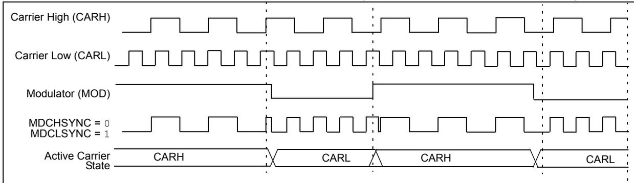
**FIGURE 22-5: FULL SYNCHRONIZATION (MDSHSYNC = 1, MDCLSYNC = 1)**
