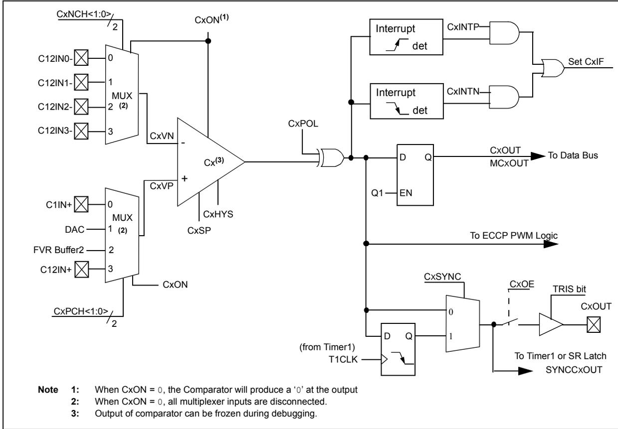
**FIGURE 18-3: COMPARATOR 2 MODULE SIMPLIFIED BLOCK DIAGRAM**
