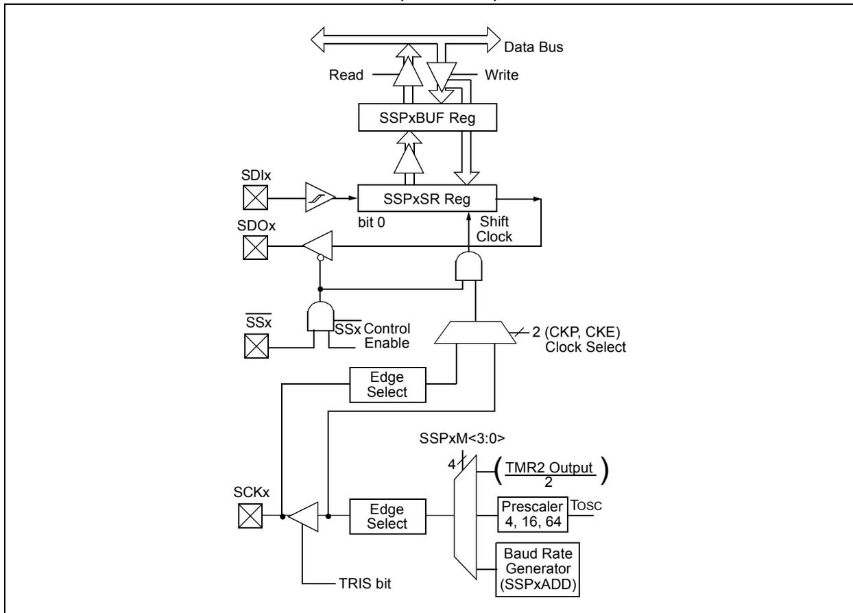
**FIGURE 24-3: MSSPX BLOCK DIAGRAM (I<sup>2</sup>C™ SLAVE MODE)**
