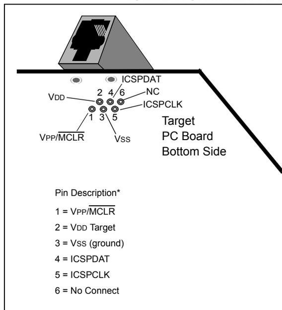
Another connector often found in use with the PICKIT™ programmers is a standard 6-pin header with 0.1 inch spacing. Refer to Figure 27-3.
