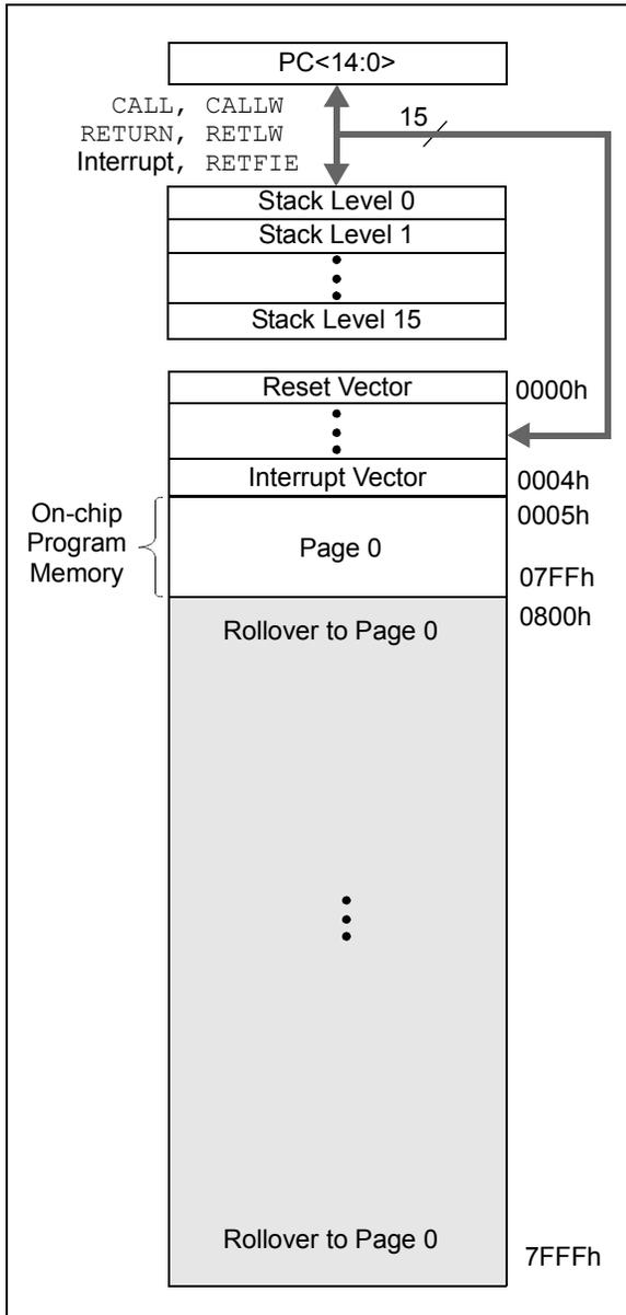
**FIGURE 3-2: PROGRAM MEMORY MAP AND STACK FOR PIC16F/LF1827**
