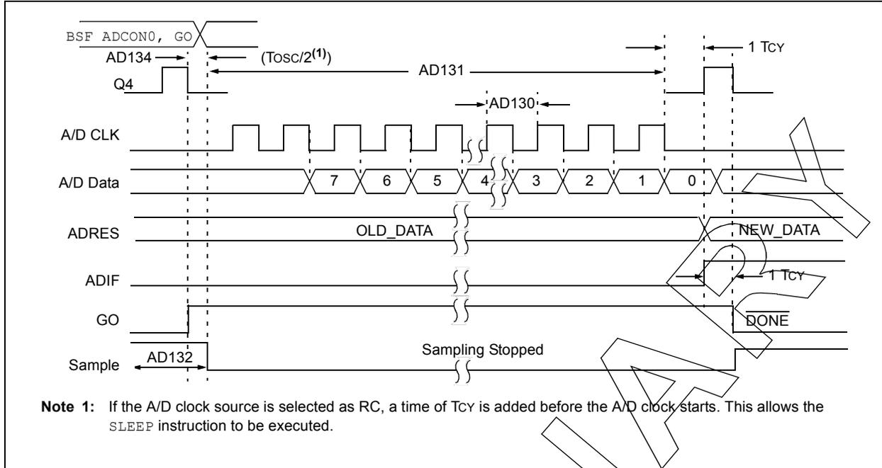
**FIGURE 29-13: PIC16F/LF1826/27 A/D CONVERSION TIMING (SLEEP MODE)**
