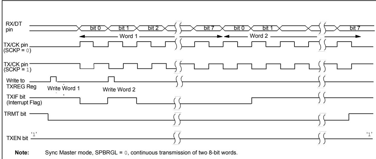
**FIGURE 25-11: SYNCHRONOUS TRANSMISSION (THROUGH TXEN)**
