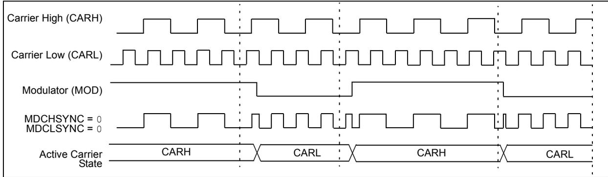
**FIGURE 22-3: CARRIER HIGH SYNCHRONIZATION (MDSHSYNC = 1, MDCLSYNC = 0)**
