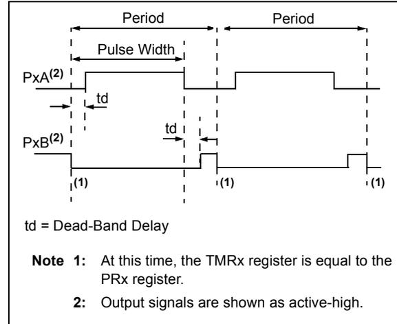
**FIGURE 23-17: EXAMPLE OF HALF-BRIDGE APPLICATIONS**
