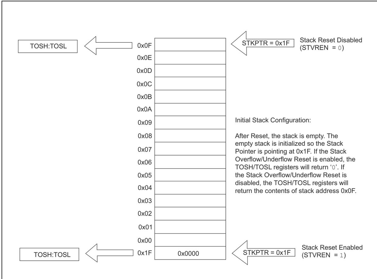
**FIGURE 3-6: ACCESSING THE STACK EXAMPLE 2**
