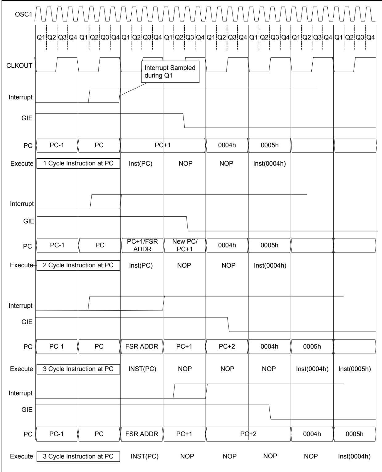
**FIGURE 8-4: INT PIN INTERRUPT TIMING**
