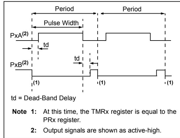
**FIGURE 23-9: EXAMPLE OF HALF-BRIDGE APPLICATIONS**
