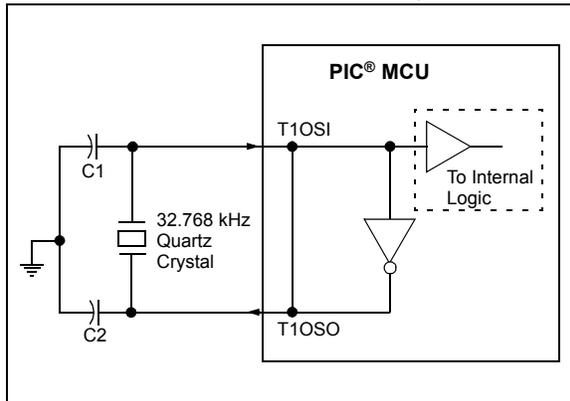
**Note 1:** Quartz crystal characteristics vary according to type, package and manufacturer. The user should consult the manufacturer data sheets for specifications and recommended application.
