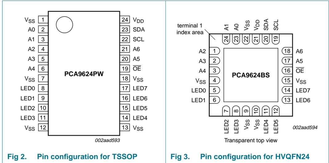
Fig 2. Pin configuration for TSSOP
