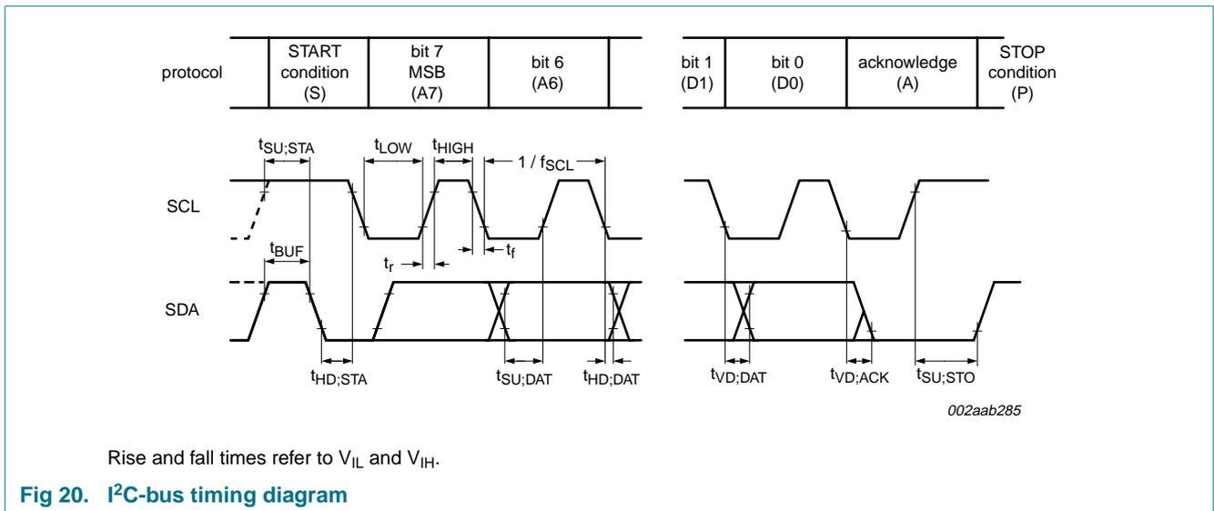
Fig 20. I<sup>2</sup>C-bus timing diagram
