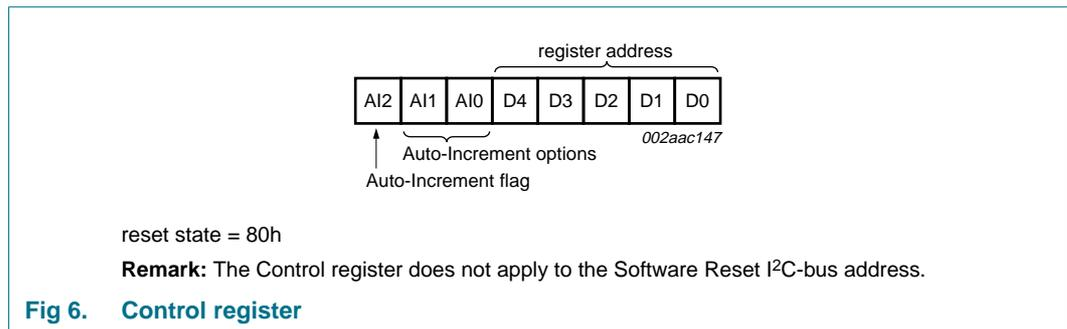
**Fig 6. Control register**
