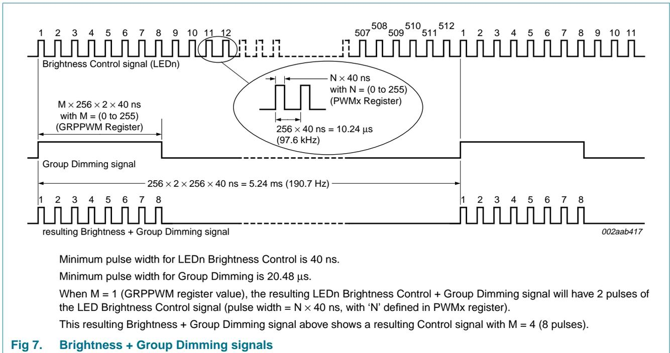
Fig 7. Brightness + Group Dimming signals
