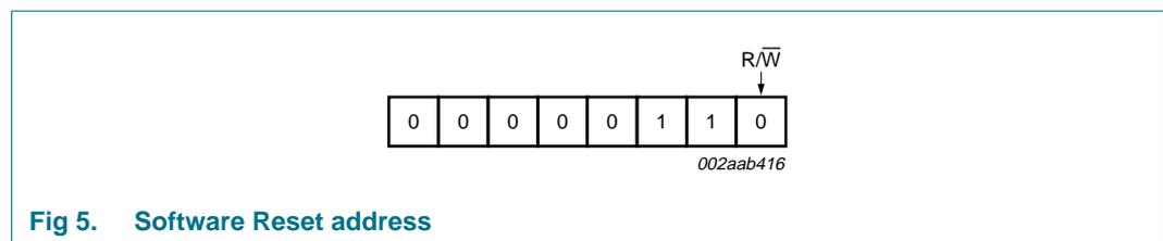
**Fig 5. Software Reset address**
