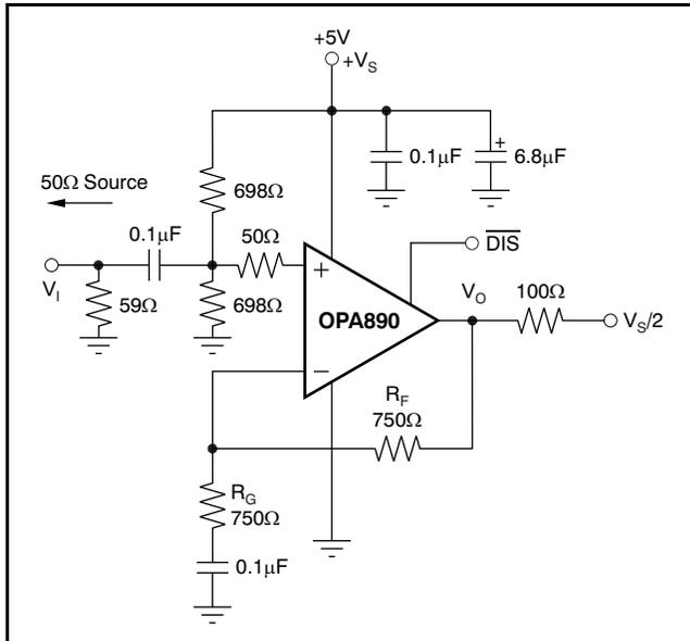
**Figure 47. AC-Coupled, G = +2, Single-Supply, Specification and Test Circuit**
