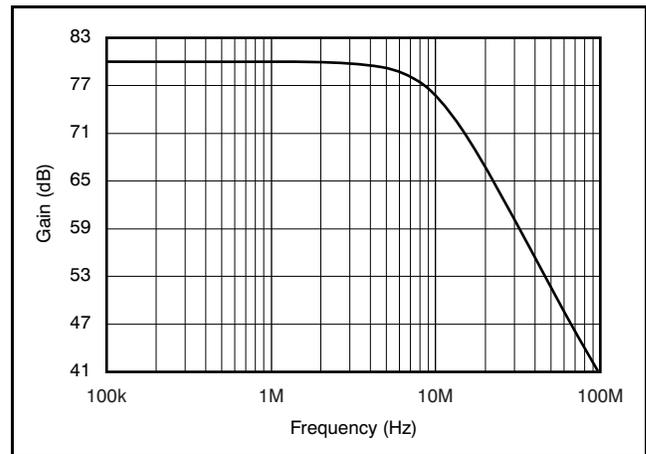
**Figure 49. OPA890 (as DAC Transimpedance Amplifier) Frequency Response**
