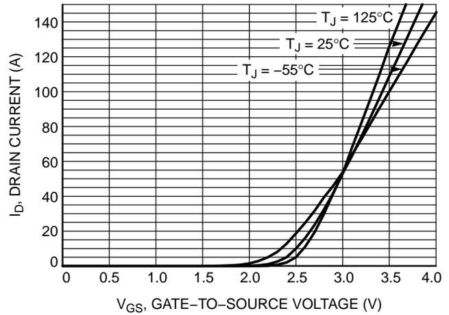
Figure 2. Transfer Characteristics
