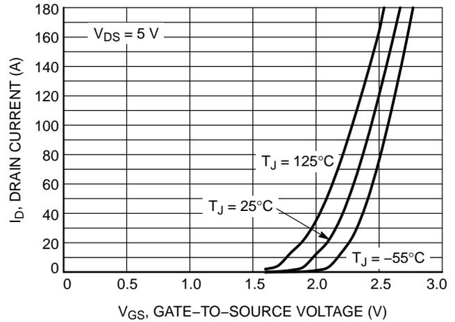
Figure 2. Transfer Characteristics
