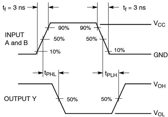
Figure 3. Switching Waveform
