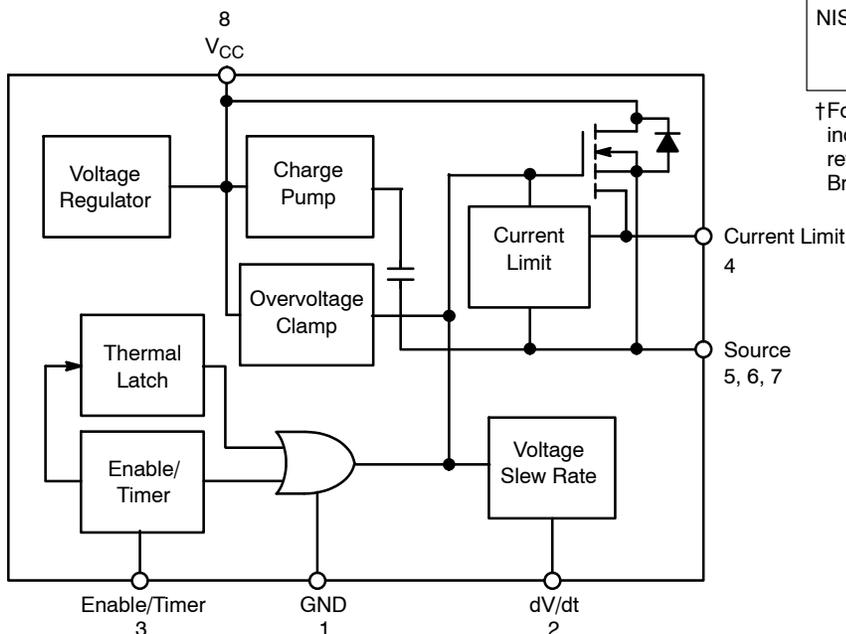
Figure 1. Block Diagram
