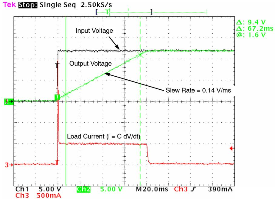
Figure 6. Turn-on Waveforms for a Load Capacitance of 3,300 μf ( $C_{dV/dt} = 1 \mu\text{f}$ )
