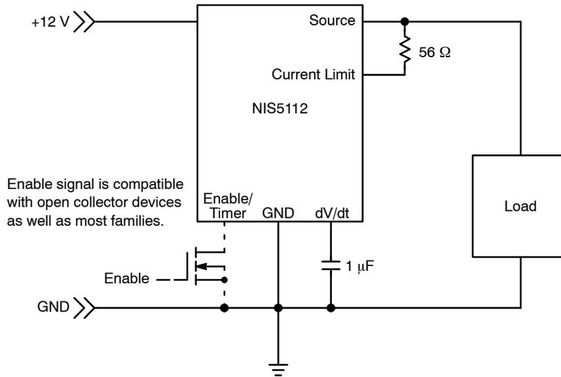
(Typical operating conditions:  $V_{in} = 12 \text{ V}$ ,  $R_{ILimit} = 56 \Omega$ ,  $C_{dV/dt} = 1 \mu\text{F}$ )
