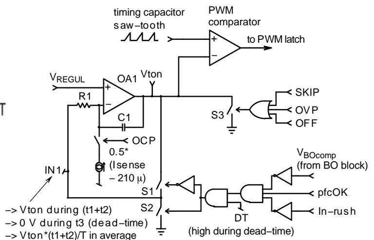
The integrator OA1 amplifies the error between  $V_{REGUL}$  and  $IN1$  so that in average, ( $V_{TON}*(t_1+t_2)/T_{sw}$ ) equates  $V_{REGUL}$ .
