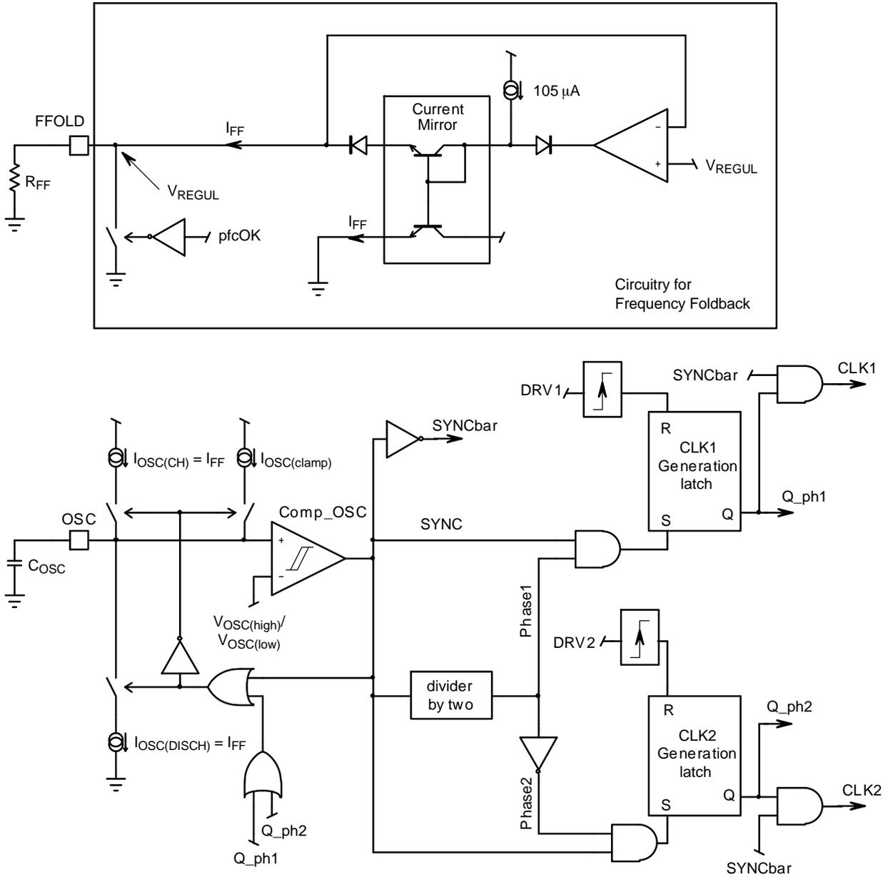
Figure 16. Oscillator Block
