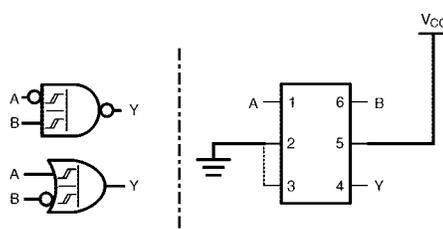
Figure 3. 2-Input NAND with Inverted A Input
