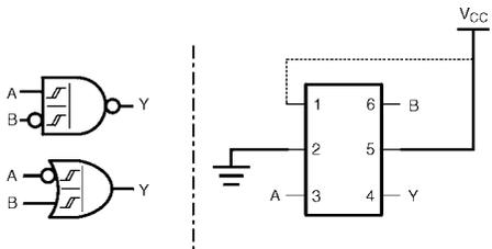
Figure 4. 2-Input NAND with Inverted B Input
