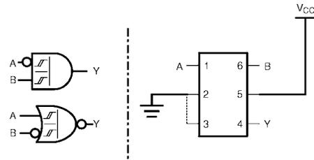
Figure 8. 2-Input AND with Inverted A Input
