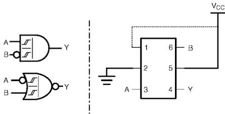
Figure 9. 2-Input AND with Inverted B Input
