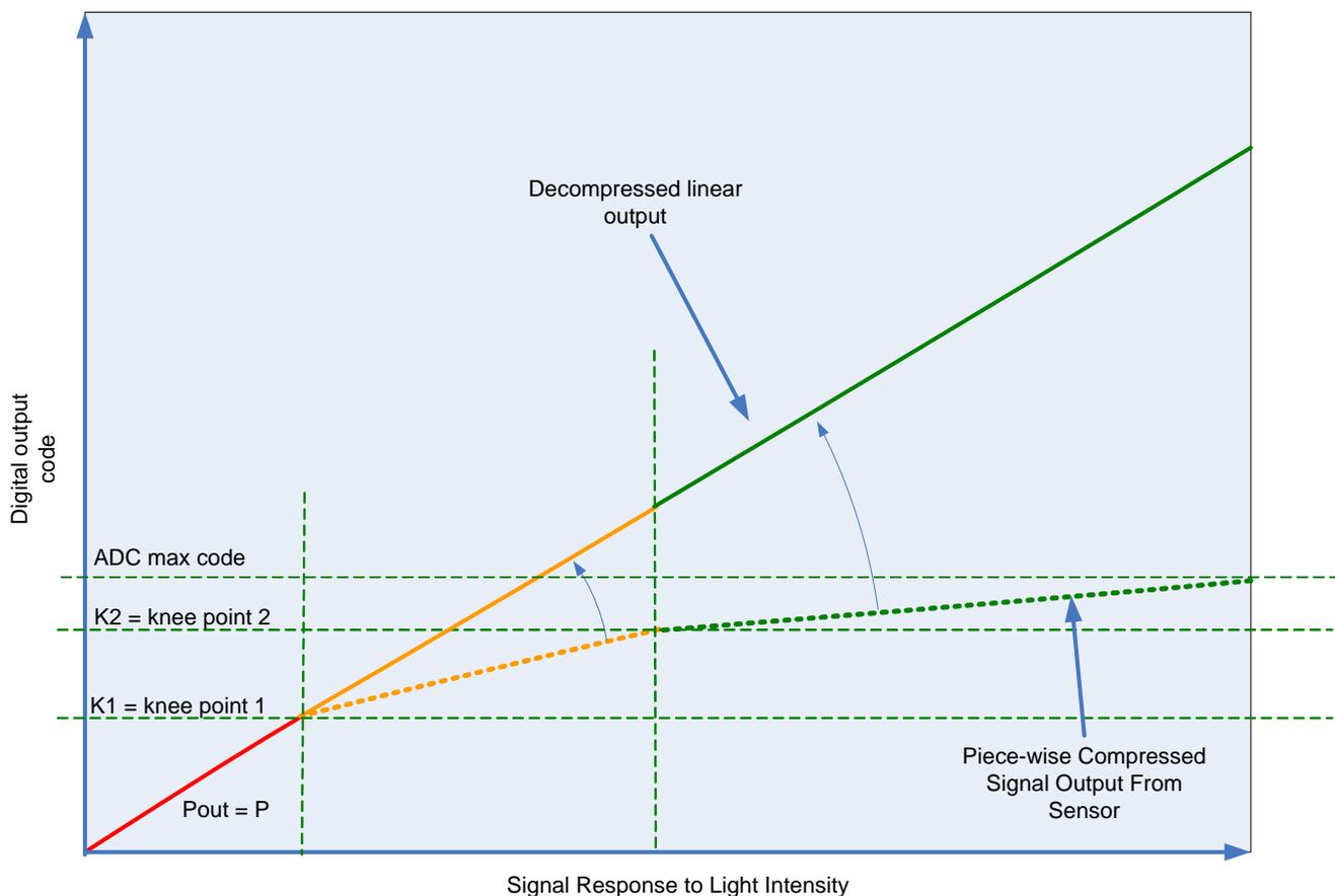
The HDR mode is selected when Operation\_Mode\_Ctrl, R0x3082[1:0] = 0. Further controls on exposure time limits and compressing are controlled by R0x3082[5:2], and R0x31D0. More details can be found in the MT9M034 Register Reference.
