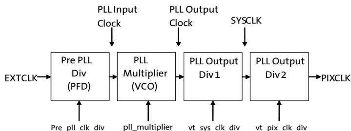
The PLL is enabled by default on the MT9M034. To configure and use the PLL:
