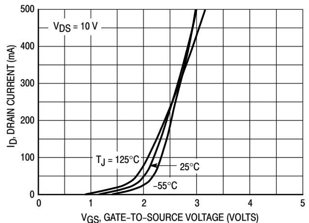
Figure 2. Transfer Characteristics
