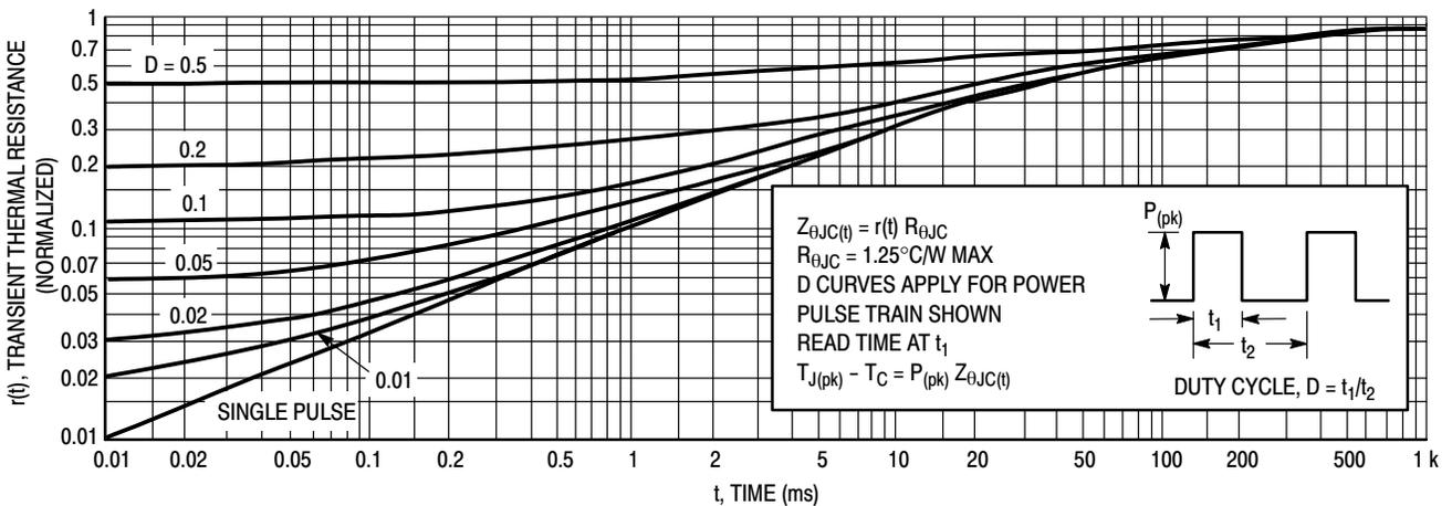
Figure 11. Typical Thermal Response [ $Z_{\theta JC}(t)$ ]
