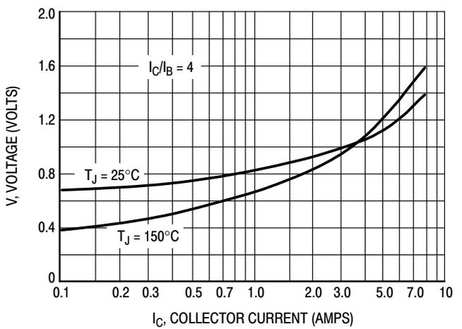
Figure 4. Base-Emitter Voltage
