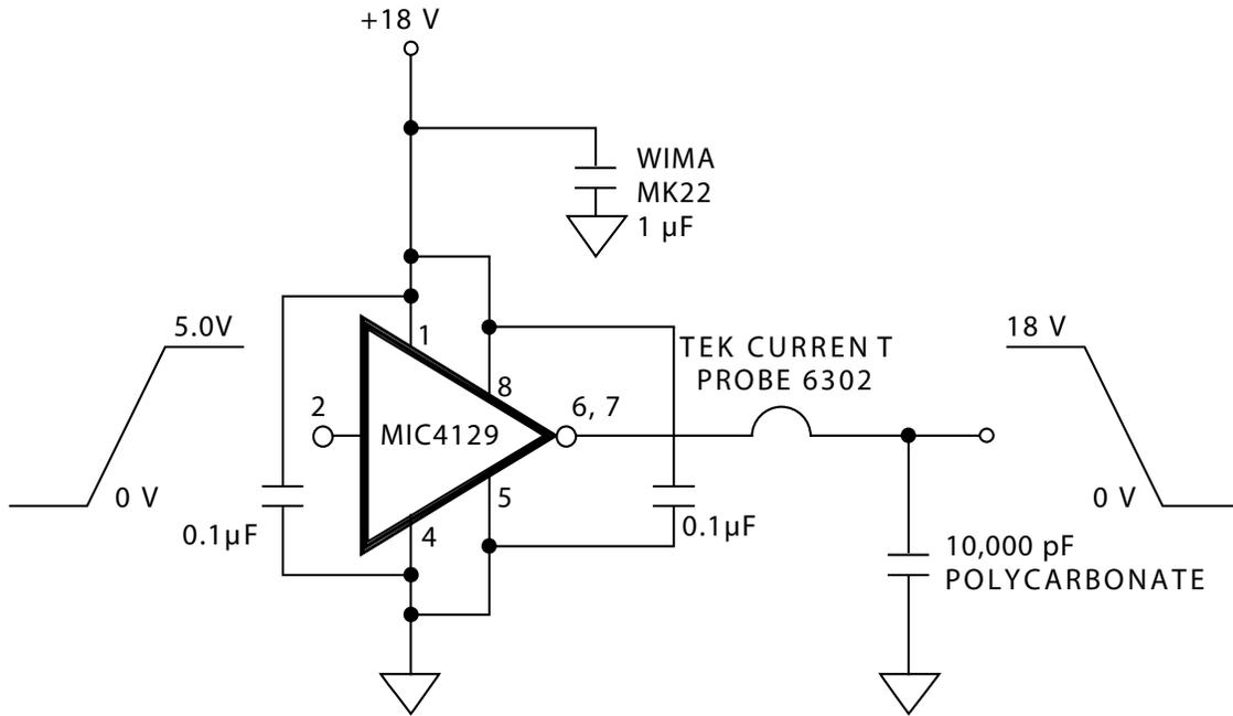
Figure 4. Peak Output Current Test Circuit
